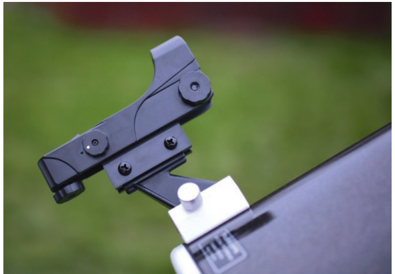
▲ The supplied red-dot finder, featuring an LED that is rather bright and needs a little toning down. Image: Steve Ringwood.
