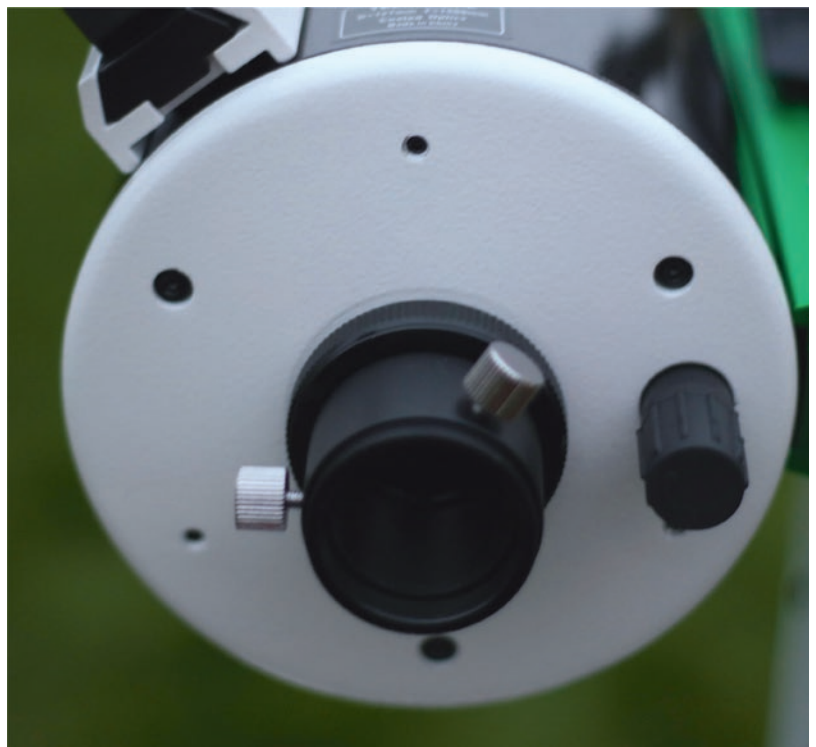
▼ The backplate, showing the combined T-mount and 1.25-inch eyepiece port and ribbed focus knob. Image: Steve Ringwood.
